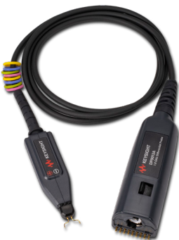
DP0013A 1.7 GHz, 42 V differential active probe
