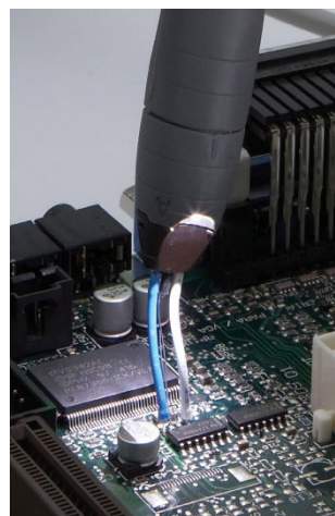
N2750A with solder-in tip
