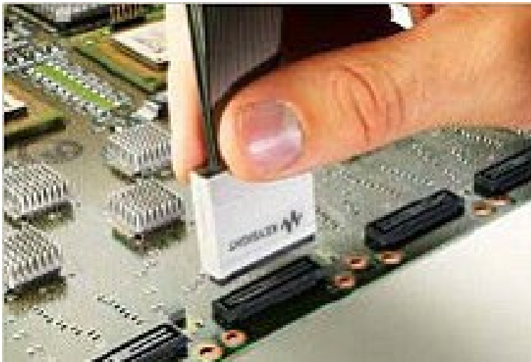
E5385A 34-channel Samtec connector probe
