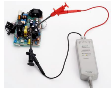
N2790A measuring a power supply signal
