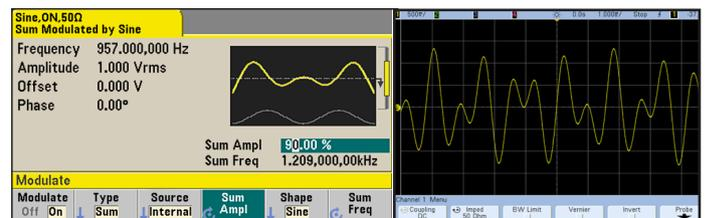
Dual-tone signal created by summing waveforms using the modulation type "Sum".
