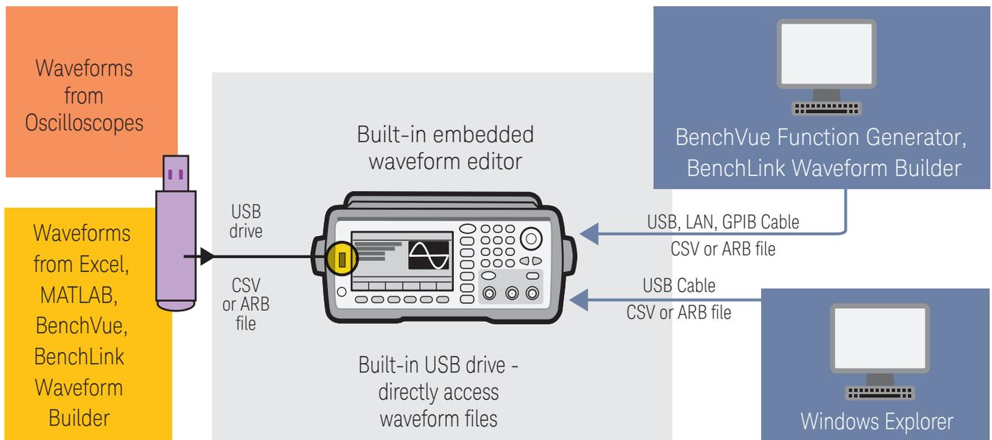
Multiple interfaces provide flexibility for creating and downloading waveforms.
