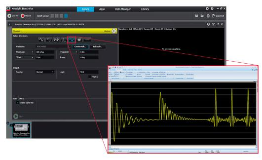
Figure 1. Design and build arbitrary waveform with Benchlink Waveform Builder Pro within BenchVue Function Generator App.
