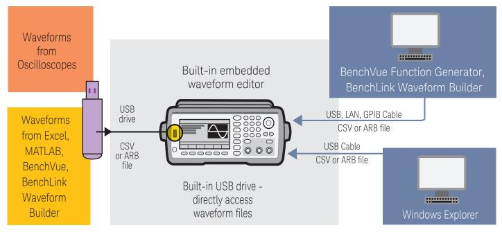
Multiple interfaces provide flexibility for creating and downloading waveforms.
