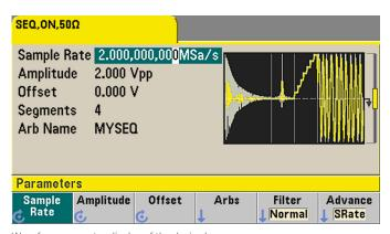
Waveform generator display of the desired sequence.
