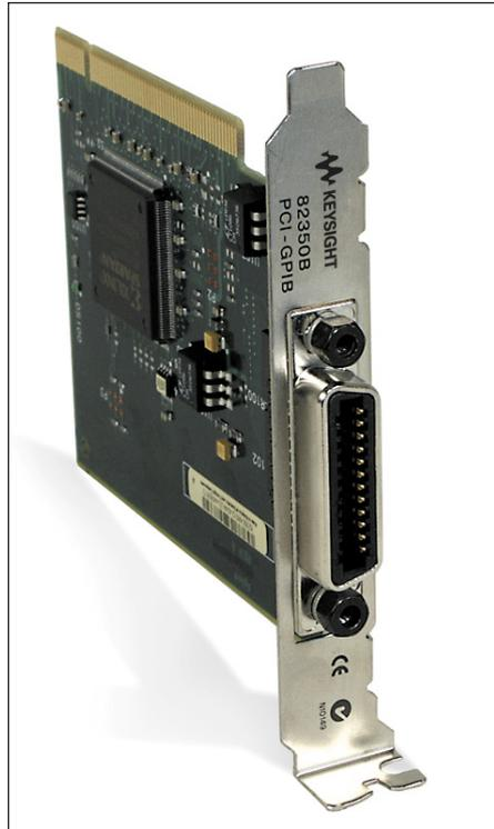
82350B PCI high-performance GPIB interface card
