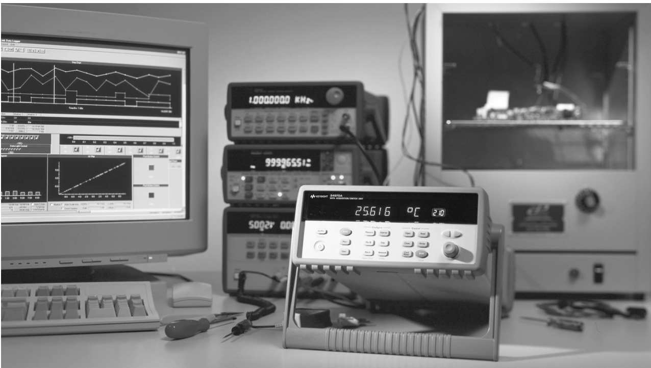
Compact 60-channel data acquisition system
