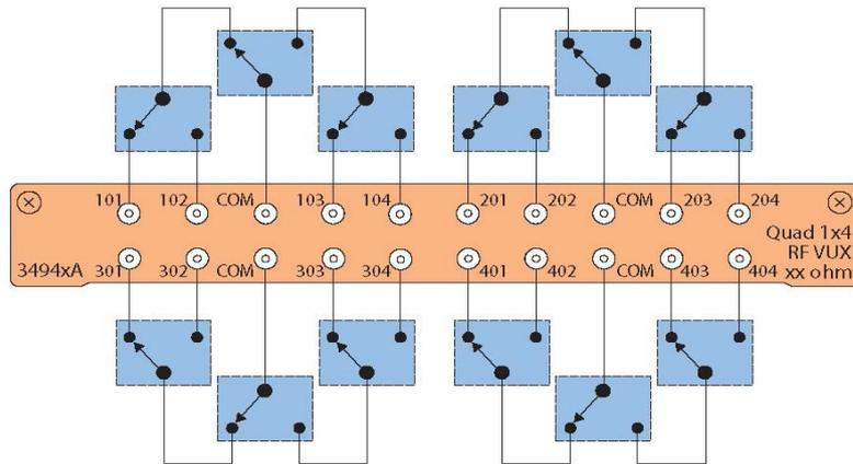
Figure 8: 34941A Quad 1x4 50 ohm 3 GHz multiplexer
