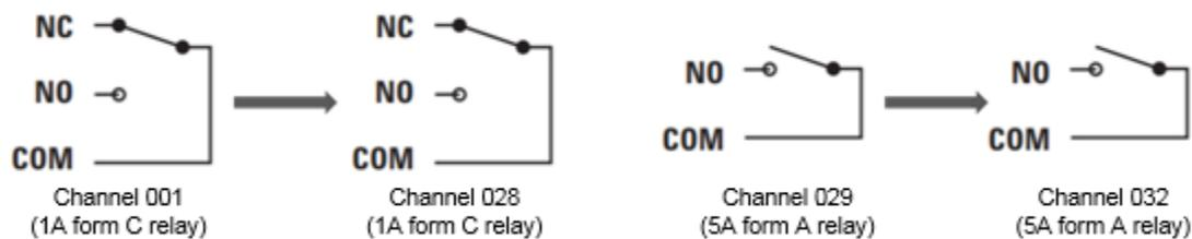
Figure 7:34937A 32-channel Form A / Form C
