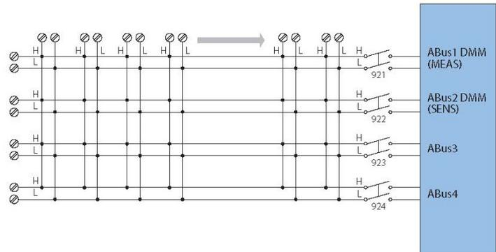
Figure 5. 34932A dual 4x16 armature matrix
