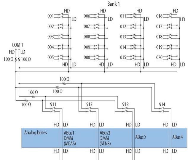
Figure 4: 34923A 40 channel reed multiplexer (bank 1 shown)
