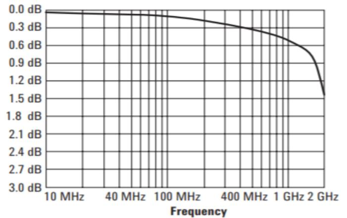
Figure 14: 34942 typical initial insertion loss
