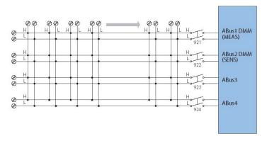
Figure 5. 34932A dual 4x16 armature matrix
