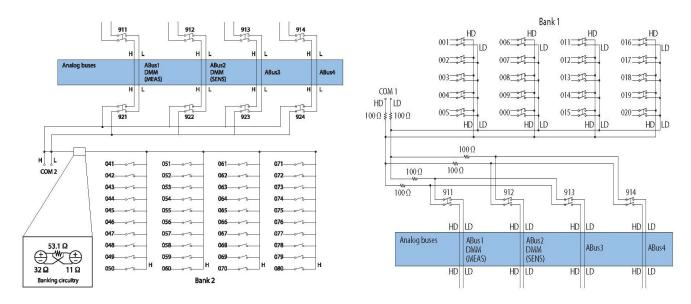
Figure 3: 34925A 40/80-channel optically isolated FET mux (shown in 1-wire mode
