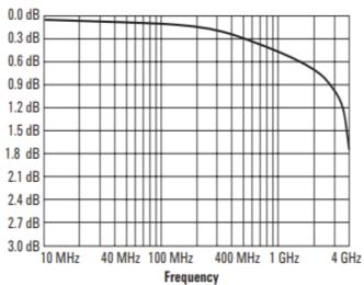
Figure 10: 34941A typical initial insertion loss
