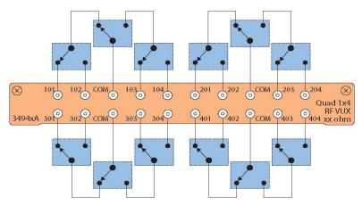
Figure 8: 34941A Quad 1x4 50 ohm 3 GHz multiplexer
