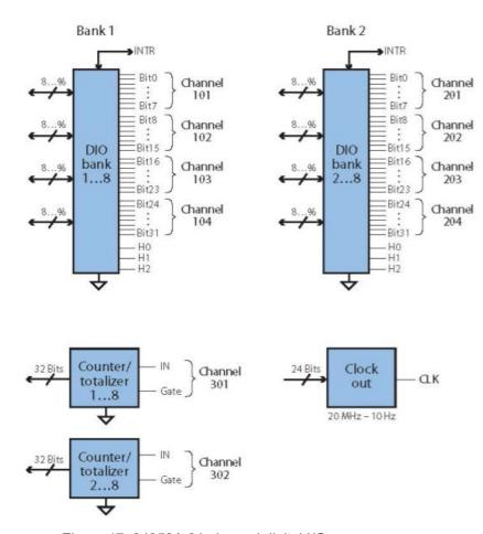
Figure 17: 34950A 64-channel digital I/O
