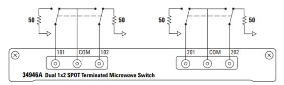
Figure 15: 34946A dual 1x2 SPDT terminated microwave switch
