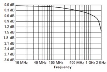
Figure 14: 34942 typical initial insertion loss
