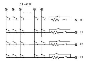
Figure 6: 34934A quad 4x32 matrix (1 of 4 matrices shown)
