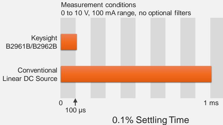
Figure 3. Fast settling time than conventional DC sources
