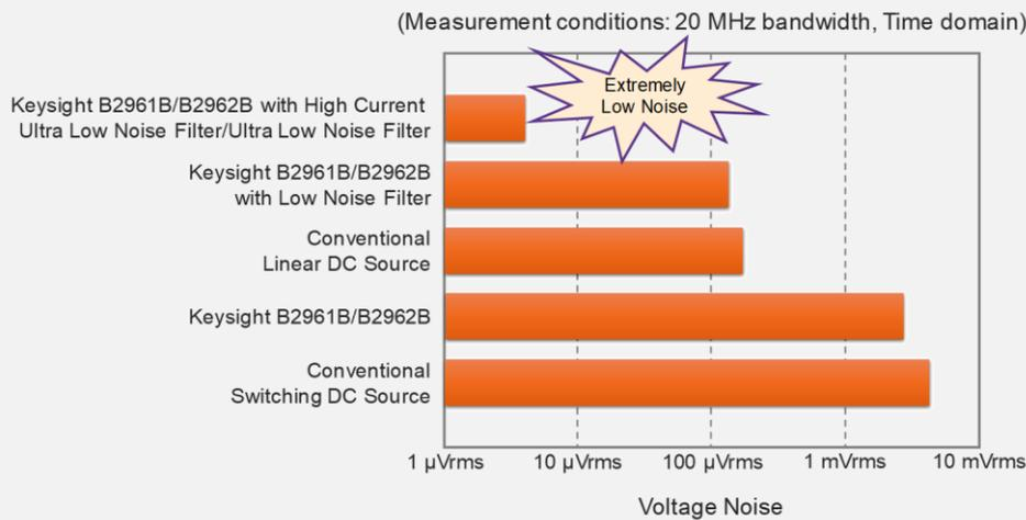
Figure 5. HC-ULNF and ULNF dramatically reduce output noise
