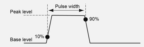
Maximum pulse width and duty cycle
