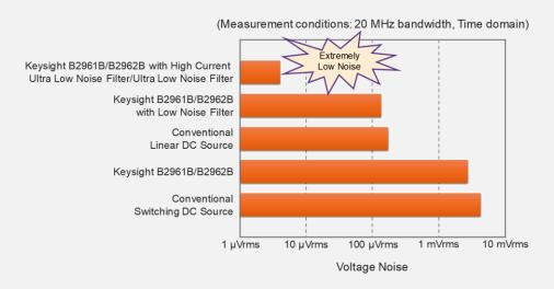
Figure 5. HC-ULNF and ULNF dramatically reduce output noise
