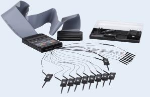
The I6-channel color-coded logic probe consists of two eight-channel pods. To make contact with the DUT, the probe connects directly to square pins or clips to test points using the included grabbers. With an input capacitance of only 8 pF and 100 k $\Omega$  input impedance, the probe protects the integrity of your signal. The probe is included with MSO models.
