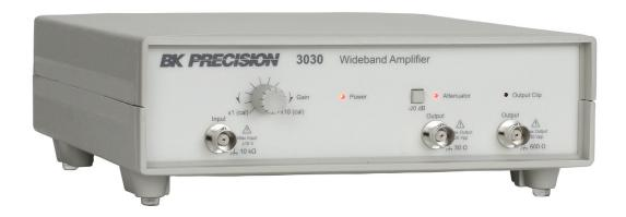
The 3030 is a DC to 1MHz amplifier with a maximum output of 30 volts peak to peak from a 50  $\Omega$  source impedance. A 600  $\Omega$  output is also provided. The unit can output up to 15 volts peak to peak into a 50  $\Omega$  load and can drive up to 300 mA peak into a low impedance or short circuit.
