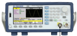
Arbitrary waveform from front panel channel output
