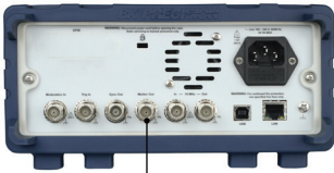
5 V TTL signal output from rear Marker Out connector
