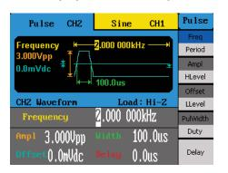
The large 3.5" color display highlights the currently selected channel and shows all relevant parameters with a preview of the waveform being generated.
