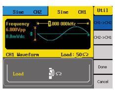
Quickly copy all waveform parameters between channels via the Utility menu. This feature can help you save time when you need to set up two identical output signals.
