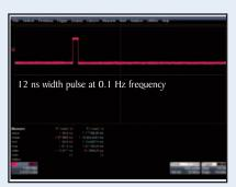
Unlike traditional DDS generators, the 4060 Series has the capability to output a rapid pulse at very low frequencies. Duty cycle can be set to as low as 0.0001%.
