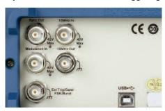
Use the external 10 MHz clock input and output to synchronize your signals to a master time base. The Sync output generates a TTL pulse for synchronization to a channel's frequency. An external trigger BNC connector is also available for inputting or generating a trigger signal.
