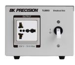
The optional TLBBS3 breakout box simplifies AC line connection between the power meter and the DUT, and eliminates the need to cut the power cord and strip wires to connect to the power meter. This breakout box supports easy plug in connection and uses a universal socket to support most plugs used worldwide. A circuit breaker/ switch is also provided for additional protection.
