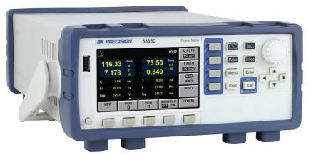
The 5335C is a compact, single-phase AC / DC power meter for measuring and analyzing power consumption and power quality parameters quickly and accurately. It supports power measurements up to 600 Vrms and 20 Arms, with a bandwidth up to of 100 kHz.
