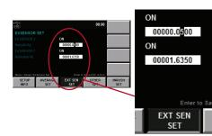
To accommodate commonly available current sensor types, users can select from the 50 mV - 2 V or 2.5 V - 10 V ranges.
