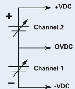
This feature is useful for powering bipolar circuits and devices.
