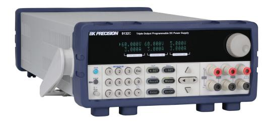
The 9130C Series triple output linear programmable DC power supplies feature isolated outputs that can be adjusted independently or combined in series or parallel to output higher voltage or current. Additionally, these supplies can operate in tracking mode with user-configurable ratios between channels.
