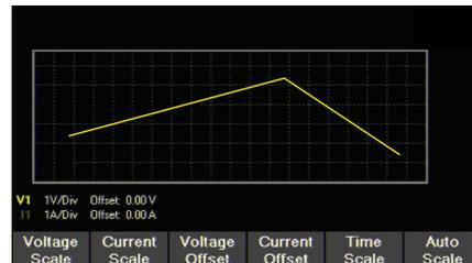
These power supplies offer a graphical display mode to visually monitor measured voltage and current data.
