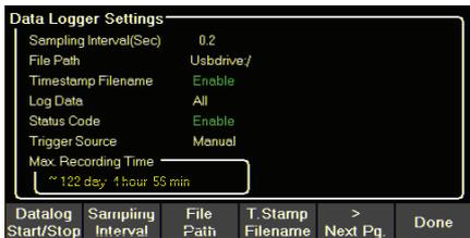
Log voltage, current, or both at a user-defined sampling interval adjustable from 0.2 seconds to 5 minutes directly to an external USB flash drive. Data points are saved as a CSV file with date and time stamp.
