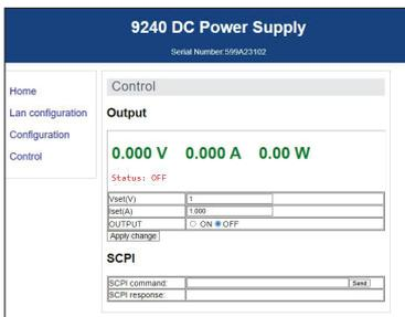
The 9240 Series provides a built-in web server that allows users to configure and control basic power supply settings from a web browser on a computer.
