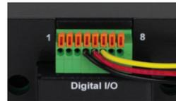
The 8-pin digital I/O terminal block preserves commonly used signaling pins including remote inhibit, AC on, and fault out capabilities while in 3-phase operation.
