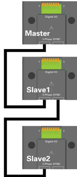
The TL983P adapters connect to the Digital I/O connector on the rear of the AC source. Standard RJ45 communication cables connect each adapter to route the 3-phase synchronization signal from the master to the slave units.
