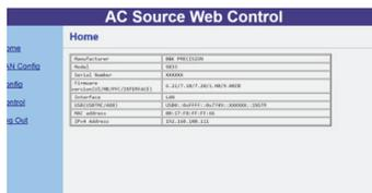
Built-in web server that allows users to configure, control, or monitor the basic settings of the power source from a remote computer using a web browser.
