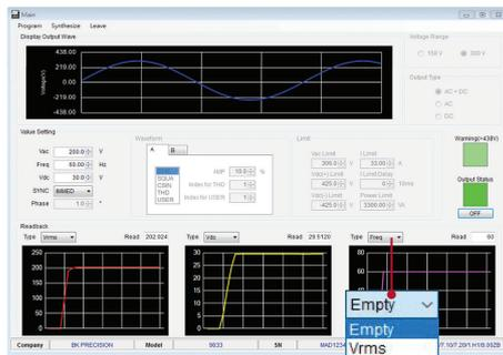
PC software is provided for front panel emulation, generating and executing List, Step, and Pulse modes, and logging measurement data without the need to write source code.
