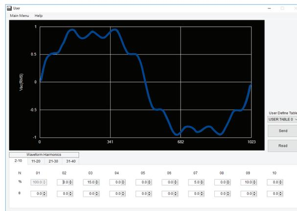
Create harmonic waveforms by specifying the amplitude and phase of each harmonic up to the 40th order.
