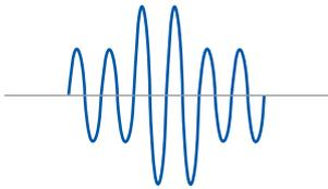
Pulse mode allows the generation of single or multiple pulses with user defined voltage, duty cycle, and phase. Either AC or DC (-424.0 to +424.0 V) output operation is supported.
