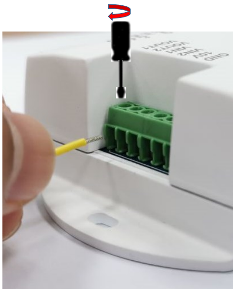
Figure 6 - Clamping wire with screwdriver in Clock-wise Direction
