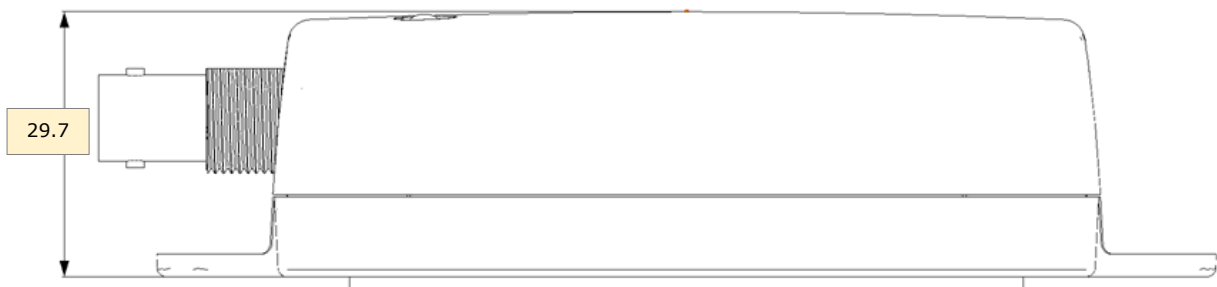
Figure 7 - Modbus EC Sensor Adapter Dimension – Side View
