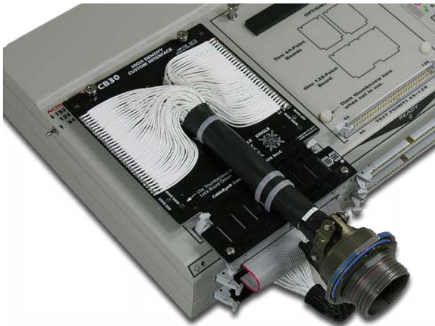
Connector Panel for Custom PLC Connectors and Flying Leads
