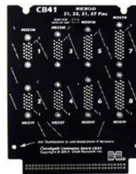
CB41 and CB41A Micro and Nano D Connectors, 21-, 25-, 31-, 37-Pin (Item 771 and 771A)
