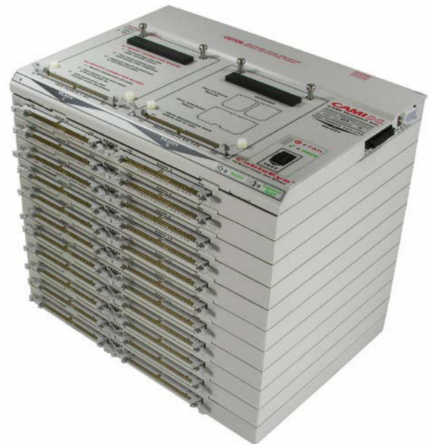
M3Z and M4 128 Test Points per Module Expandable to 2560 TP
