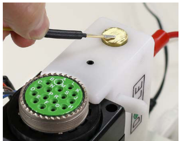
ZIF Block with Integrated Probe Plate
