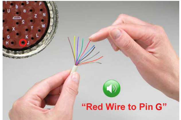
AutoBuild™ Guided Assembly with Speech Setup for 2nd-Sided pinning with Electrical test. Target pin highlighted and read aloud. (Item 728)
