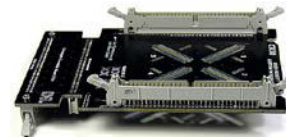
Side View of CB30 with 64-Pin Headers Attached (headers not included)
