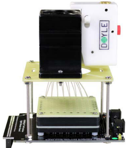
Side View Showing Fibers Entering Mating Connector
