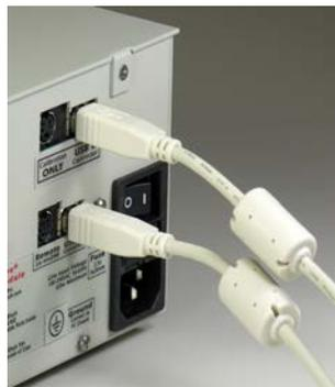
Picture 1: USB cables with ferrite core
