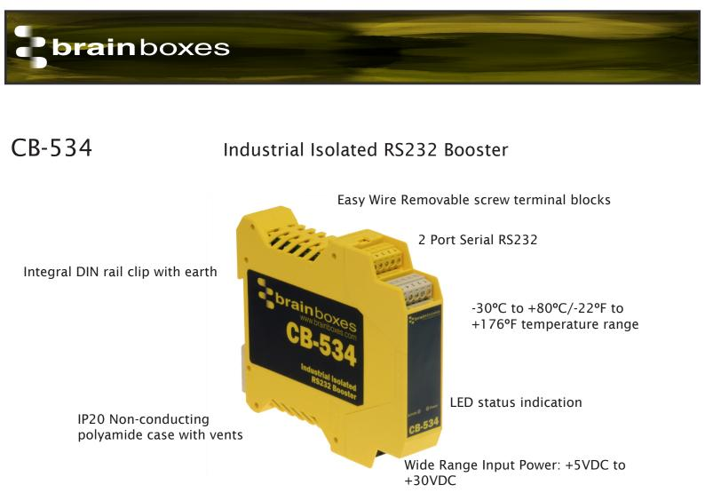
Booster for RS232 signal can extend cable length. Works with a wide voltage swing and outputs -11V to +11V signal making it suitable for legacy and non-conforming RS232 equipment. Provides isolation between two RS232 devices. This product doesn't require any software, simply connect using the easy-wire numbered terminal blocks.
