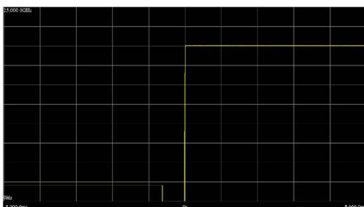
The 1435 series signal generator can realize fast frequency switching in the full frequency band, and the measured frequency switching time is  $0.67\text{ms}$ , which can meet the test requirements for high speed.
