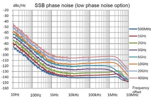
The 1435 series signal generator provides two steps of phase noise for users. The standard phase noise is measured at  $-101\text{dBc/Hz}$  ( $10\text{GHz}@10\text{kHz}$ ), and the phase noise can be as low as  $-116\text{dBc/Hz}$  ( $10\text{GHz}@10\text{kHz}$ ) when the low phase noise option is selected. Users can select the phase noise as required to achieve the optimal cost performance.
