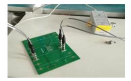
By using the automatic fixture removal function, the measured parts are taken as a whole to extract the balance parameters and to implement 4-port embedded. The test results show that the transmission parameters can be removed well including the near-end and far-end crosstalk.
