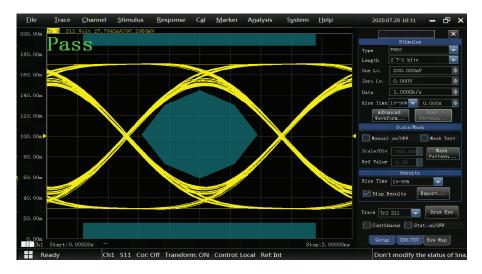
The advanced time-domain analysis option can impose jitter, noise and other interference on the simulation eye map, and simulate the simulation eye map of different positions of high-speed link in the real environment through the addition of correction algorithms such as pre-weighting and equalization.
