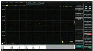
Parameters can be entered quickly by using the activated input toolbar. Set limit line and segment scan value for production line to improve test efficiency.
