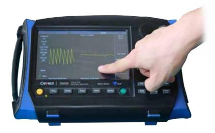
The 7 measurement types can be switched by finger sliding, no need of menu operation.
