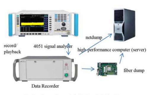
RF signal streaming and playback analysis function
