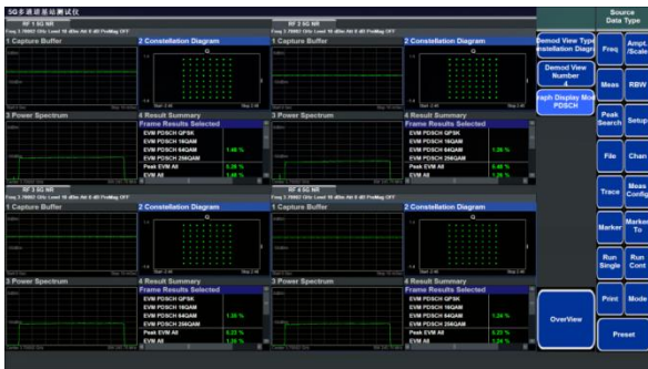
Multi-channel Test for 5G NR Base Station Signal (100 MHz BW)
