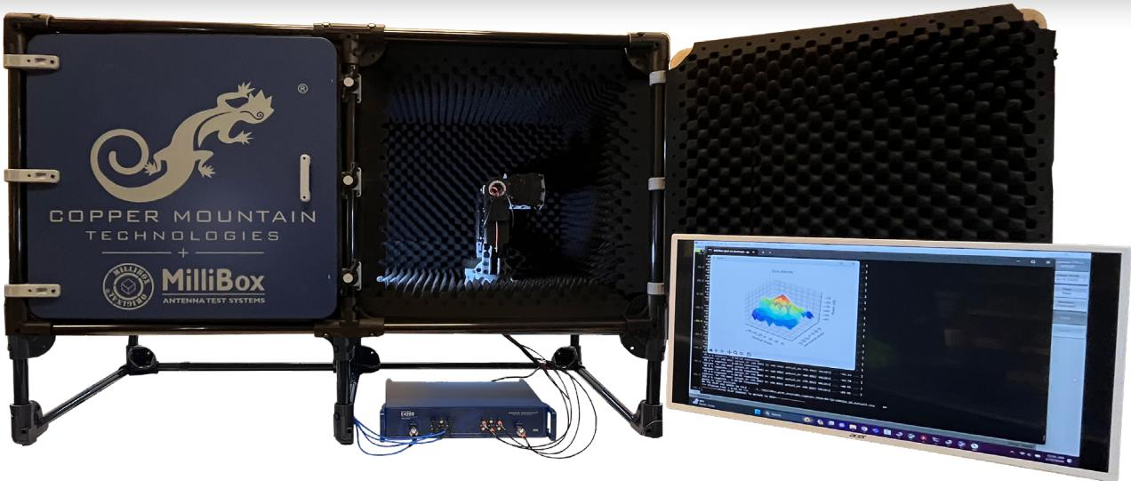
A new turnkey solution for customers needing to make far-field and sub-THz antenna measurements for bands from WR-15 to WR-05. The over-the-air (OTA) antenna test system features a wide array of configurations depending on the user's far-field requirements, antenna size, desired frequency range, and antenna positioner functionality.
