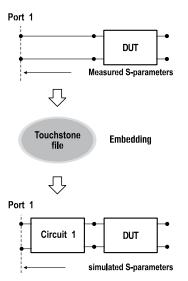
Allows the user to mathematically simulate the DUT parameters after virtual connection through a fixture circuit between the calibration plane and the DUT. This circuit is described by an S-parameter matrix in a Touchstone file.
