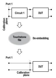
Allows users to mathematically exclude from the measurement result the effect of the fixture circuit connected between the calibration plane and a DUT. This circuit should be described by an S-parameter matrix in a Touchstone file.
