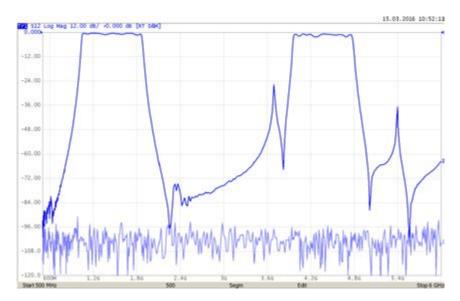
The 162 dB dynamic range of Cobalt VNAs combined with high measurement speed per point allows measurement of SAW filters' S-parameters with full 2-port calibration and 1601 measurement points in less than 32 ms while still maintaining more than 100 dB measurement range (IFBW at 1 MHz). This measurement speed corresponds to the performance of the most advanced handlers used for automatic verification of mass-produced SAW filters.
