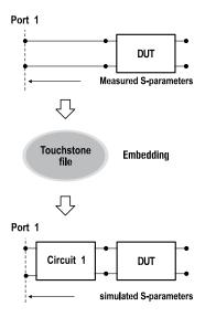
Allows the user to mathematically simulate the DUT parameters after virtual connection through a fixture circuit between the calibration plane and the DUT. This circuit is described by an S-parameter matrix in a Touchstone file.
