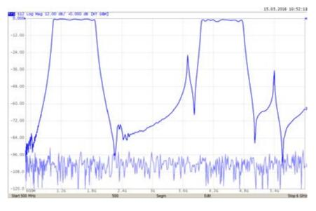
The 135 dB dynamic range of Cobalt VNAs combined with high measurement speed per point allows measurement of SAW filters' S-parameters with full 2-port calibration and 1601 measurement points in less than 32 ms while still maintaining more than 85 dB measurement range (IFBW at 1 MHz). This measurement speed corresponds to the performance of the most advanced handlers used for automatic verification of mass-produced SAW filters.
