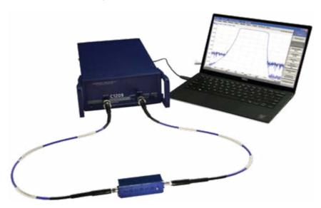
Cobalt 20 GHz VNAs have 135 dB dynamic range at 1 Hz IFBW, which allows them to maintain a wide measurement range at high measurement speeds. Measurement of all S-parameters of a BTS filter with full two-port and 801 measurement points with 1 MHz IFBW takes only 17.5ms while maintaining a measurement range of over 85 dB. This time is almost completely determined by the IFBW of the VNA. This measurement speed allows for real time tuning of high isolation BTS filters.
