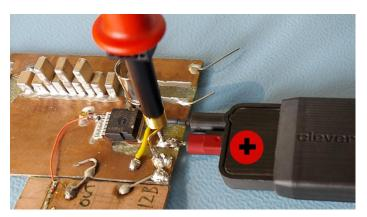
Here 0.64mm square sockets have also been used to simultaneously measure  $V_{\text{DS}}$  with a x200 probe
