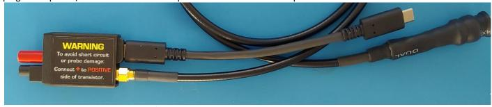
Connect the other end of the power/control cable to the Isolator. Connect the 8 pin Mini Din cable to the CS448 LINK PORT and the internally terminated (500hm) and insulated coax cable to a CS448 channel input.
