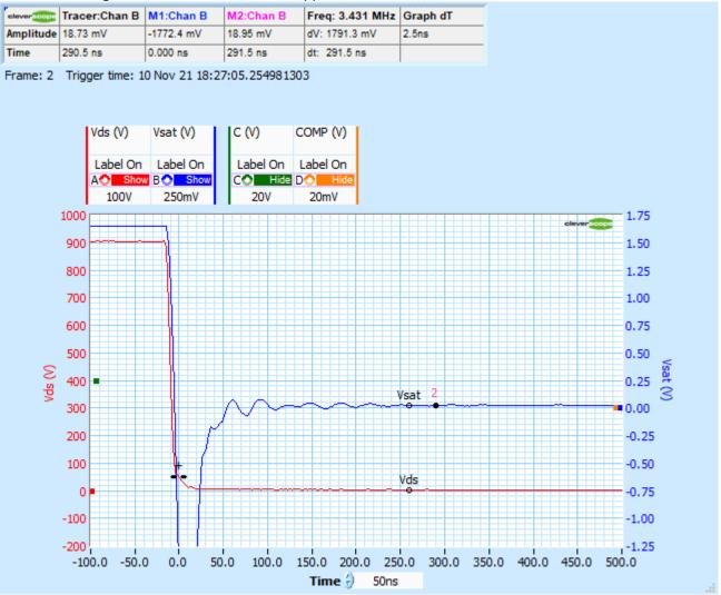
Flatness on the 1.5V range over 500us is about 1.6 mV (M1-M2). The 37mV voltage drop is due to the approx 1 Ohm on resistance of the FET with the 30mA current source through it, and the uncorrected CS1133 offset:
