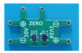
The Calibrator will be used by the updated Cleverscope 4 application to precision calibrate the CS1133. Accuracy is already pretty good (1%), but the calibrator will increase accuracy to about 0.1%. A calibrator is included with each CS1133.
