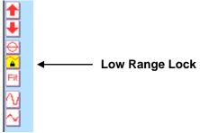
Note: If you leave the button locked, the CS448 will clip signals greater than the low range maximum value (probe dependant). If this happens, unlock the range.
