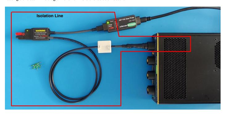
All items within the isolation line (Channel A, Probe Head, Coax cable and output of Isolator) have a common reference connection which will be connected to the UUT Source (or Emitter). If the Source is a high side transistor in a half bridge this whole isolation island will move with the switching edges of the half bridge. A common mode choke (as supplied with the CS448) may be required on the coax cable to suppress common mode induced spikes and ringing.
