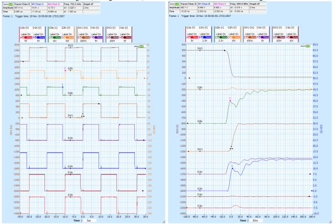
Zoom in on the PDF. Measure the dead time (Marker 1 to Marker 2, 1.383us in this example), the Miller plateau, check for Miller induced droop, Miller induced gate voltage bumps, and use the Maths to measure Gate charge etc.
