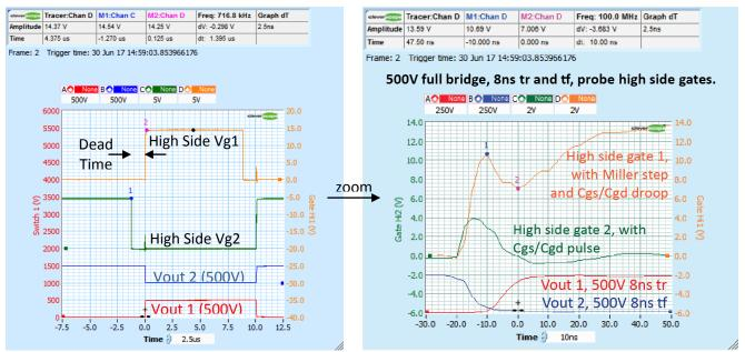
The high CMRR, and the isolation allow the high side gate drives to be measured without large common mode artifacts. We can observe dead time, pulse timing, the gate charge characteristic, and parasitics such as the Cgs/Cgd droop and pulse effects.
