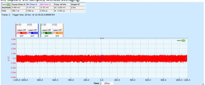
We use the signal information display to calculate the Standard Deviation (a good estimate of RMS, less the DC) and the peak to peak. We see about 200uVrms noise, and less than 1.8mV p-p noise.
