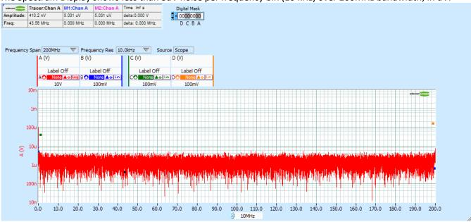
The Spectrum Display shows less than 8uV noise per frequency bin (10 kHz) over 200MHz bandwidth, in uV:
