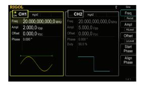
Two channels with complete equivalent functions and precisely adjustable phases (standard)
