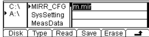
All the configurations (system and sensor configuration) can be cloned into other DM3058/DM3058E on product line via USB storage device to improve work efficiency.
