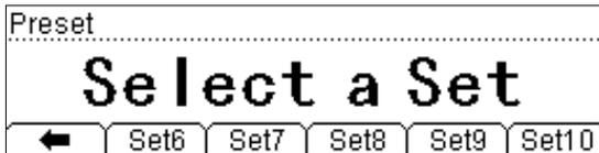
Based on Preset Mode, the worker operation on product line could be greatly simplified. Besides, 10 groups of Preset Configuration are available to be stored and recalled.
