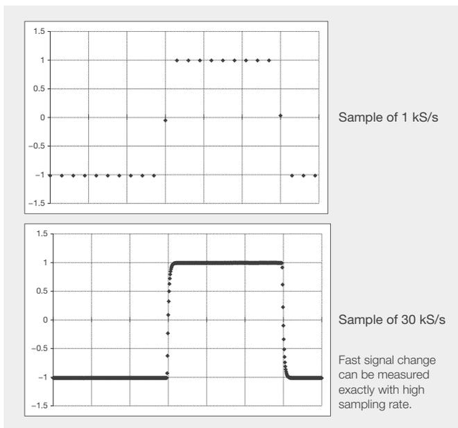
Setting the DM7560 to 30 kS/s enables users to see the details of a 10 ms pulse width on a 2 Vpp measurement.
