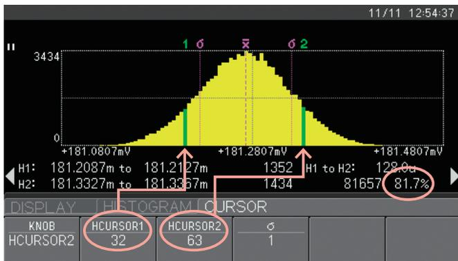
Yield rate and other calculations are available using cursor controls on the histogram display.
