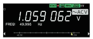
Numerical value + Frequency + Analog meter Users can display the input signal voltage and frequency side-byside with numeric values and indicators.
