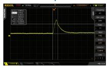
The transient response time is less than 50  $\mu$ s. When the transient change occurs to the load current, the output voltage can be quickly restored to the set value, ensuring the output quality.
