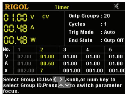
When the timing output is enabled, the system will configure the voltage, current, and the duration time based on the preset timer parameters, so as to provide varied voltage and/or current output for the load.
