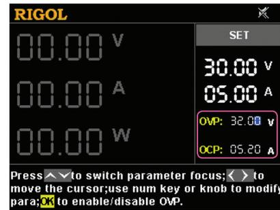
You can set thresholds for OVP and OCP values. If overvoltage or overcurrent occurs, the power supply shuts down the output automatically, and then a prompt message is displayed.
