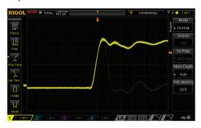
UltraVision: waveform recording and playback functions
