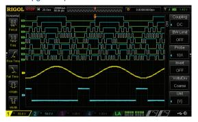
UltraVision: up to 30,000 wfms/s waveform capture rate
