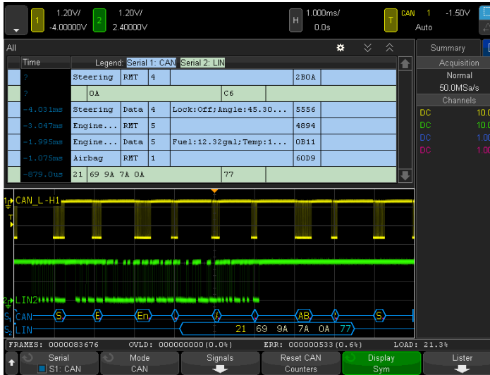
Figure 20. Dual serial bus CAN and LIN decode and interleaved “lister” display.
