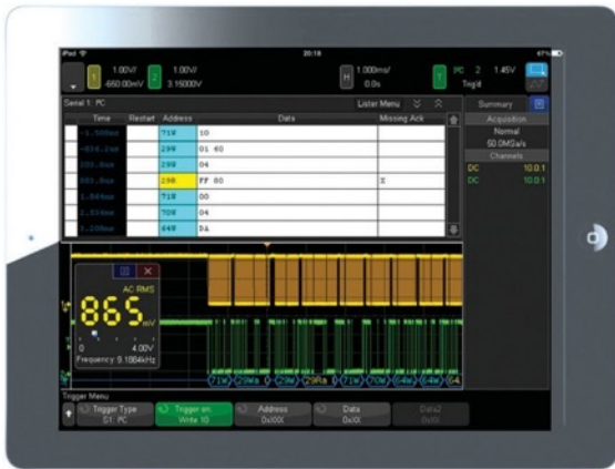
Figure 37. Tablet virtual front panel control.
