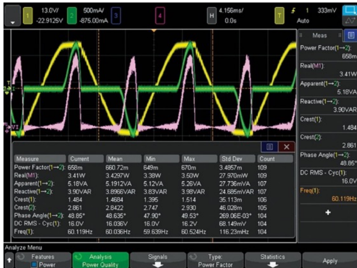
Figure 26. Power quality measurement, one of many in the power measurements application.
