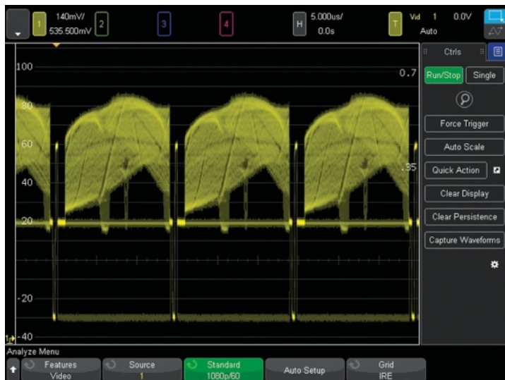
Figure 27. Triggering on 1080p HDTV signal analysis.
