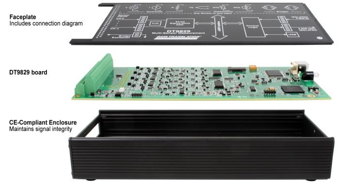
Exploded view – the DT9829 case packages the DT9829 in a CE-compliant enclosure
