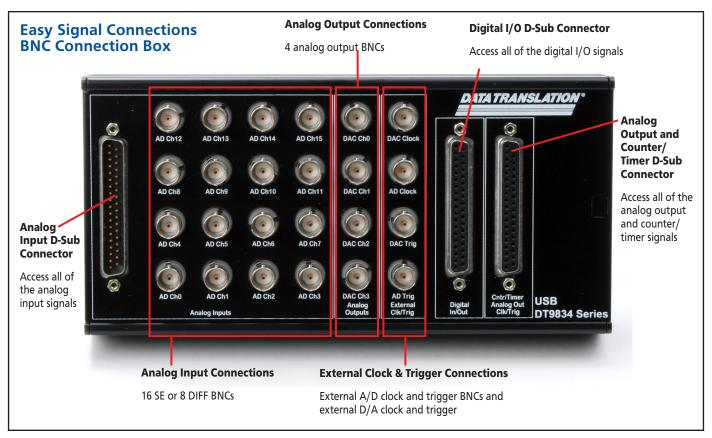
The BNC connection box is available for easy signal connections.
