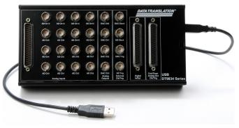
DT9834 Series modules are available in two configurations: BNC connection box and OEM embedded version.
