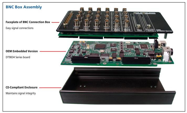
The BNC connection box packages the OEM embedded version of the DT9834 Series in a CE-compliant enclosure.
