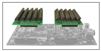
The EP355 screw terminal panel plugs into the J2 or J3 connector of a DT9834 Series module.
