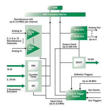
The DT9836 and DT9832 Series provides USB 2.0 multifunction modules for simultaneous operation of analog input, analog output, digital I/O, and counter/timer subsystems.
