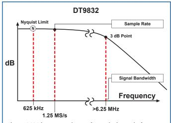
The DT9832 has a sample rate for each channel of 1.25 MS/s. This means that the Nyquist limit allows signal frequencies up to 625 kHz to be adequately measured. The analog input components have a signal bandwidth that is ten times the Nyquist limit or in this case, greater than 6.25 MHz to minimize roll-off and phase errors.
