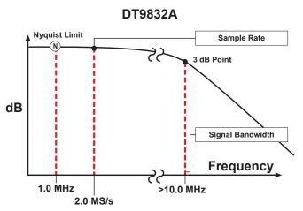
The DT9832A has a sample rate for each channel of 2.0 MS/s. This means that the Nyquist limit allows signal frequencies up to 1.0 MHz to be adequately measured. The analog input components have a signal bandwidth that is ten times the Nyquist limit or in this case, greater than 10.0 MHz to minimize roll-off and phase errors.
