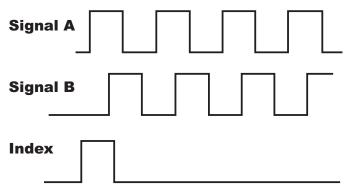
A quadrature decoder takes the output signals (A, B, and Index) for the quadrature encoder as inputs and converts these signals into a numerical value that can be used to determine position, distance, velocity, and other functions.
