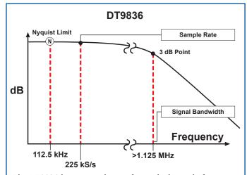
The DT9836 has a sample rate for each channel of 225 kS/s. This means that the Nyquist limit allows signal frequencies up to 112.5 kHz to be adequately measured. The analog input components have a signal bandwidth that is ten times the Nyquist limit or in this case, greater than 1.125 MHz to minimize roll-off and phase errors.
