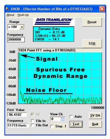
These graphs show the outstanding quality of the DT9832 Series and DT9836 Series for all error sources with ENOB (Effective Number Of Bits) ratings of 13.6, 13.6, and 14.1 bits respectively and an SFDR (Spurious Free Dynamic Range) of 86 dB to 95 dB.
