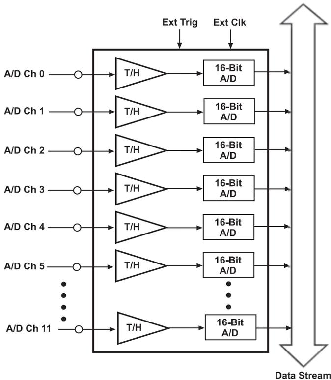
*The DT9836 Series features 6 or 12 independent, successive-approximation A/D converters with track-and-hold circuitry. Each converter uses a common clock and trigger for simultaneous sample of all analog inputs at 225 kS/s per channel. The DT9832 Series features 2 or 4 simultaneous A/D converters with sample rates up to 2.0 MS/s.*
