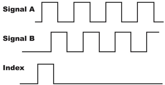
*A quadrature decoder takes the output signals (A, B, and Index) for the quadrature encoder as inputs and converts these signals into a numerical value that can be used to determine position, distance, velocity, and other functions.*
