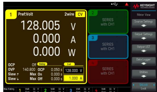
Figure 3: Increase output voltage with E364SNP kit.
