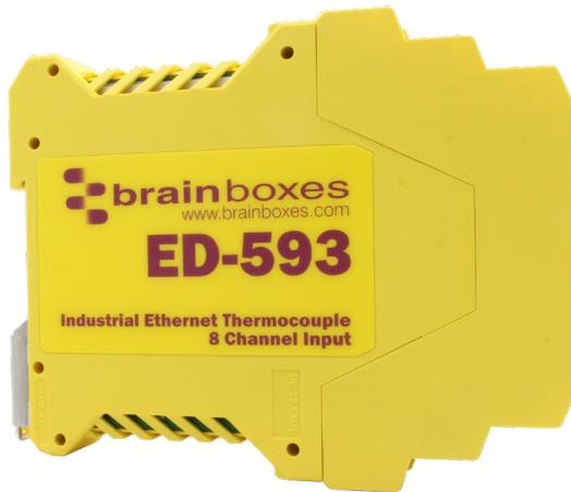
IP20 non-conducting polyamide case with vents
